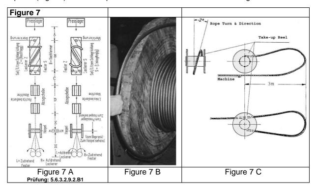
**Turns in strands** depending on Type of lay and rope/strand construction. In regular lay ropes depending on strand construction between 1 and 4 opening turns. Lang lay construction require closing (tightening) turns in strands ½ to 1 ½. Rope should have 0-Turns with a very light tendency of closing (tightening)
