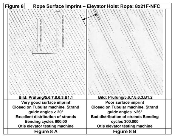
Imprint of Lay Length give the exact lay length and shows if strand clearances are even.
